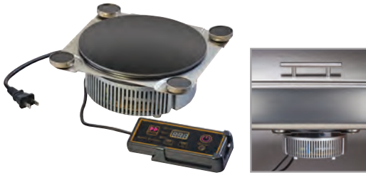
I. MAGNETIC INDUCTION CHAFER ATTACHMENT Converts Chafers with Easy Access Drawers into Flameless Induction Units. Stainless Steel Piece is Placed in Water Pan, Unit Attaches Magnetically Below. ITEM 4011 | 8¼Wx8¼Dx3½H
